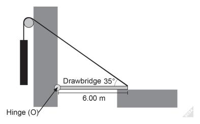
A castle has a 6.00 m long drawbridge with a mass of 500 kg over its moat. It is attached to a winch by an extremely strong rope at an angle 35.0° to the horizontal.
