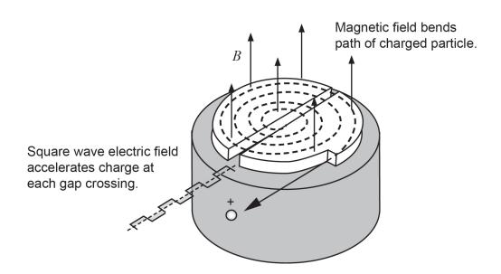
The cyclotron frequency (how often the electric field between the dees reverses) is independent of both the velocity of the particles and the radius of the circular path they follow.
