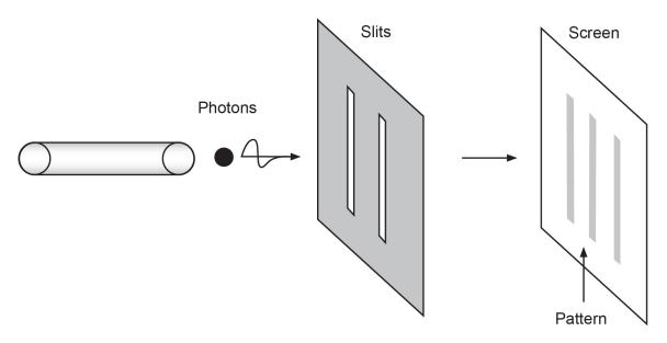
The diagram above shows that when monochromatic coherent light is shone through two narrow slits onto a screen, light and dark fringes appear on the screen.
