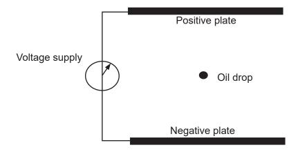
Initially there is no potential difference between the plates and the student chooses an oil drop and, using a microscope, watches as it slowly falls, measuring its speed. The student determines that the speed is constant at 0.0313 mm s<sup>-1</sup>.
