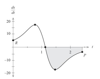
The definite integral  $\int_{a}^{b} \left(\frac{ds}{dt}\right) dt$  was evaluated so that the area for the shaded region could be determined. This area is 13.4258 square units.
