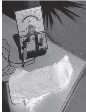
Solar cell in sunlight, with covering
