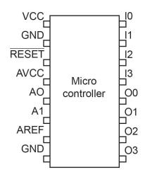
(d) The controller will use an output for a DPDT relay Y1, which will be used as a H bridge that will drive a motor M1 from a separate 10 A 24 V DC source. It will also use a SPDT relay Y2 triggered by an output to turn the motor power off and on. Draw this configuration, using the diagram below. (12 marks)
