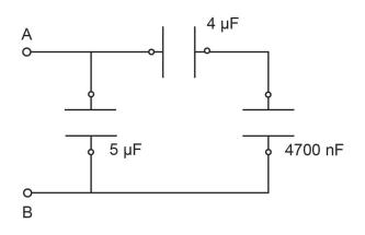
(e) Calculate the value of the capacitor required to bring the total capacitance between A and B in the circuit above to 10 μF and correctly draw it into the circuit in part (d). (2 marks)
