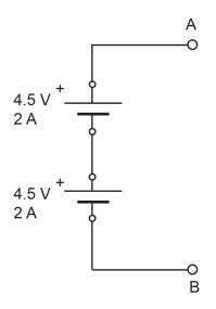
The circuit below is that of a battery pack made from two 4.5 V cells.
