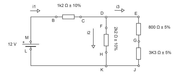
(a) Explain how you would measure the current flowing from the voltage source into the 1k2  $\Omega$  resistor. (3 marks)
