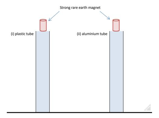
The magnet falling through the plastic tube travelled much faster than the magnet falling through the aluminium tube. Explain, clearly indicating the physics principles involved.
